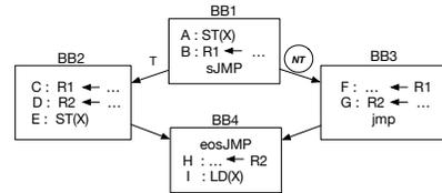
Fig. 4: Basic Blocks with Phantom Dependencies. Secure branch’s true path is not taken (NT).
