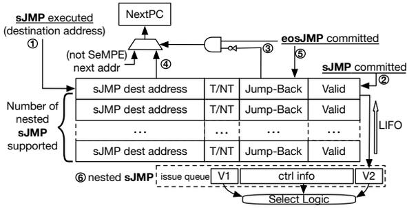
Fig. 5: Micro-architecture support for SeMPE. The branch outcome is saved in the T/NT bit field, where T is *Taken* and NT is *NotTaken*
